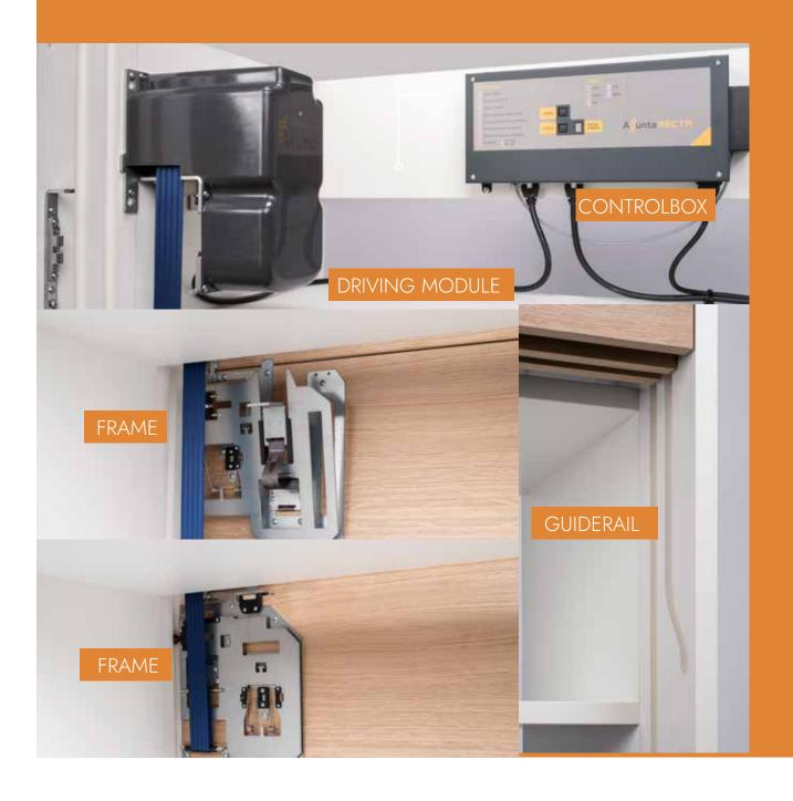
Assunta is very simple in design. The system consists of 2 drive modules, a control box and frames that are attached to the panels. The frames for the panels contain all the necessary components and are screwed onto the panel as one unit. This leads to a very simple and fast assem**bly**. The frames are different according to the panel: on the lower panel, frames come with guide wheels and attachment points for the belts. The frames for the following panels
